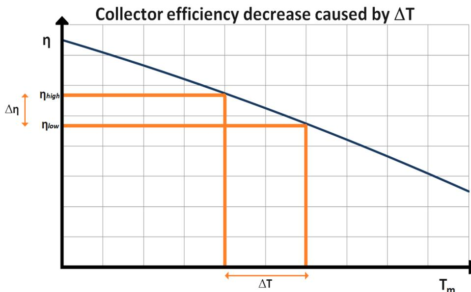
Fig. 7.4.1. Efficiency decrease caused by the temperature over the heat exchanger (difference between primary and secondary side temperature). (Source: PlanEnergi)
