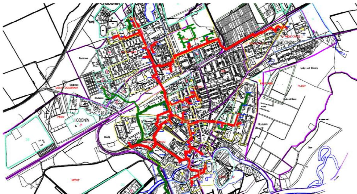
For evaluation of possibilities to implement alternative energy sources, the locality "South-East estate" has been chosen. It is an area in Southeastern part of Hodonín where primary-level as well as secondary-level transfer occurs. The area is currently connected with steam feeder Hodonín. Average heat supply to the customers is 77 165 GJ.
