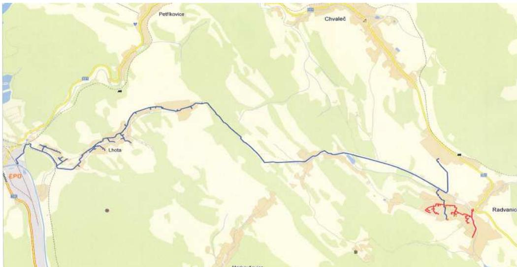
The dimensions of the steam line Radvanice corresponds with the capacity of the supply for coal mines in Radvanice. Due to the termination of mining in this locality the capacity of the steam line is excessive. That leads to higher relative heat losses of the system, particularly in Summer.
