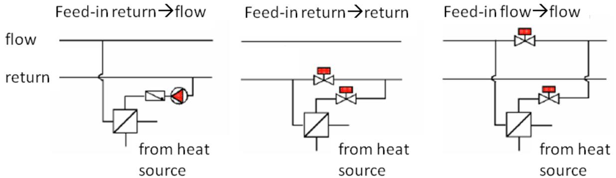
Fig. 5.2.2. hydraulic integration of solar thermal feed-in (source: Streicher)
